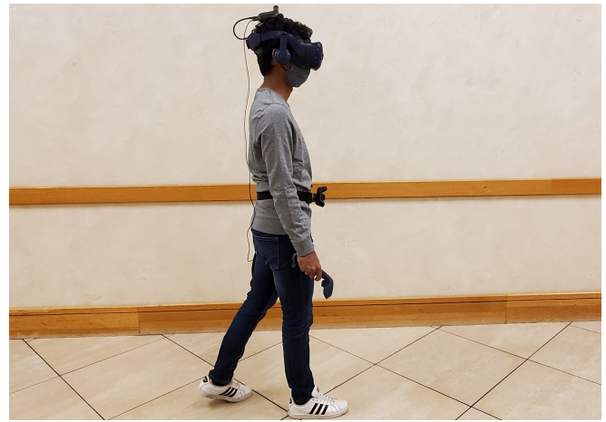
(b) Participants wear an HTC Vive Pro Eye head-mounted display with a WiGig wireless adapter and an HTC Vive Tracker on a belt mounted to the waist. They interact with controls in the experiment using the Vive Controller.
